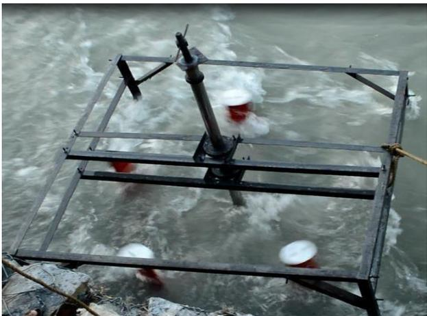
Figure 11: Testing of VAWT in shallow water channel
